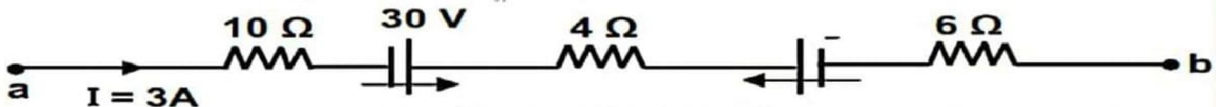
$$V_{ab} = 3 \times (10 + 4 + 6) - 30 + 10 = 40 \text{ V}$$
